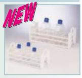
Flasks can be more easily organized to improve processing and avoid errors in collecting used medium, medium change, washing of cell monolayer, trypsinization and seeding of cells. Grips on each end make rack handling easy and allow for safe transport of flasks to the incubator. Steam autoclavable at 121°C (250°F).
